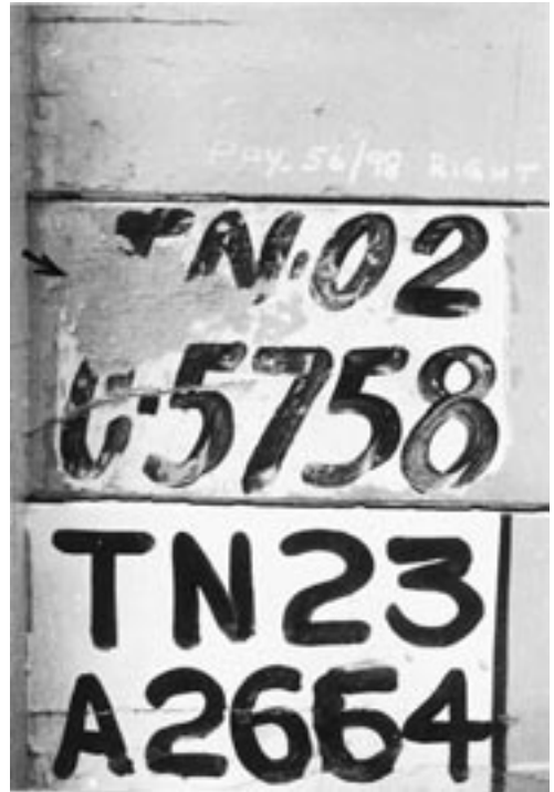
FIG. 4—The restored registration number “TN-02-C-5758” just above the existing registration number on the right rear of the lorry (see Fig. 2) (arrow mark indicates the area of erasure).
